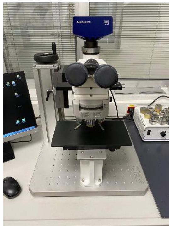
Metallographic Microscope for the measurement of the Recrystallization layer
