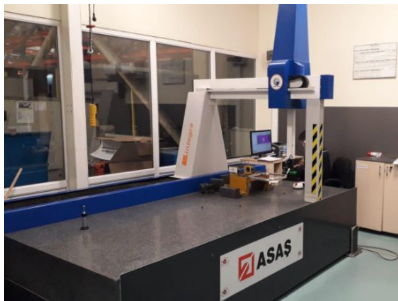
CMM (Coordinate Measuring Machine) used in ASAS for Geometric Tolerance Measurement
